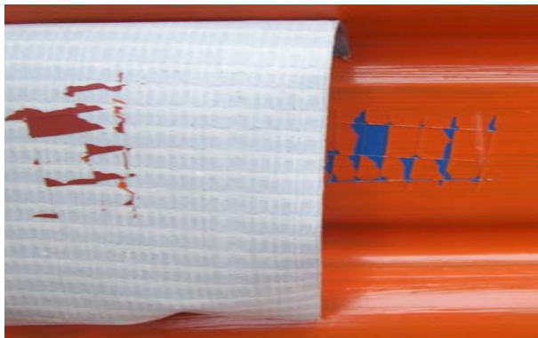
Pull Tests with Paint samples that failed.
